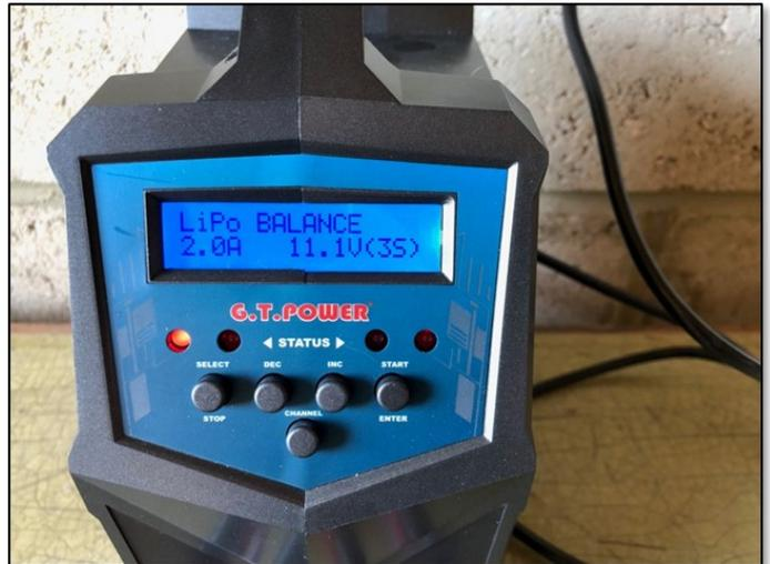
charging time down enabling me to charge 8 batteries in a couple of hours. You can mix battery types and sizes without a problem as each channel is completely independent of the others. It is in effect four chargers in a single case.
